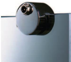
Can be mounted to glass plates, mirrors, shelves etc. up to a material thickness of 7mm/0.27". Particularly suitable for fitting our lamps on bathrooms mirrors, etc. To determine PIPE length please specify material dimension or measure center to center. ø 31mm/1.2" / h=20mm/0.8".
